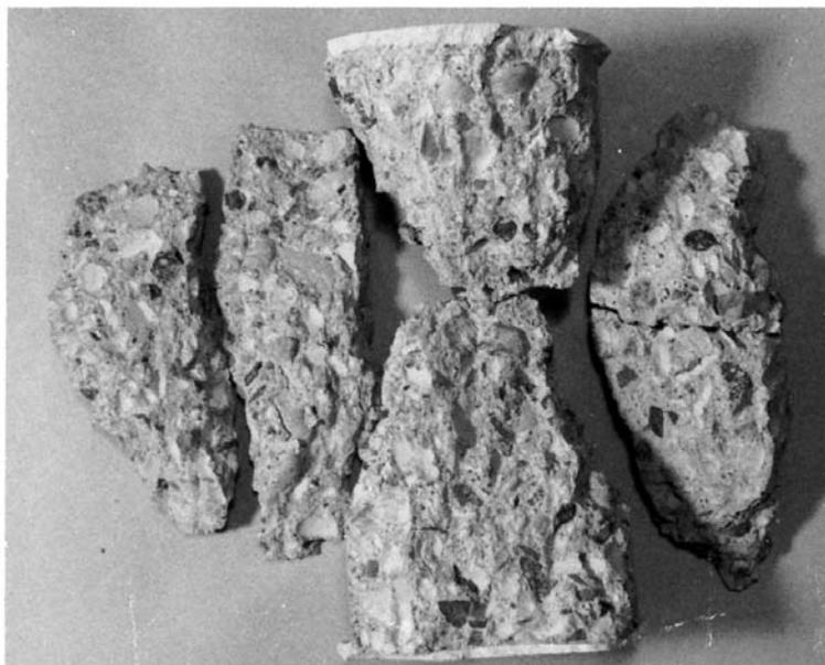
NOTE 1—Cones are usually better defined. The upper cap on this cylinder is too thick.
