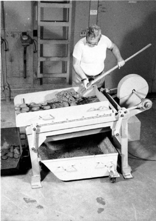
FIG. 6 Mechanical Equipment for Wet Sieving Concrete
