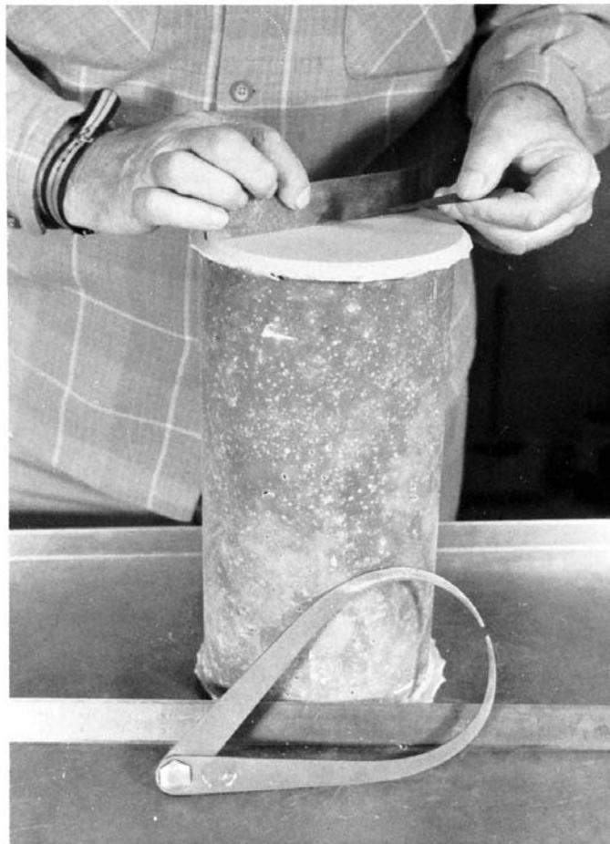
NOTE 1—The outside caliper and the scale are used to measure the diameter of the cylinder for computing the area.
